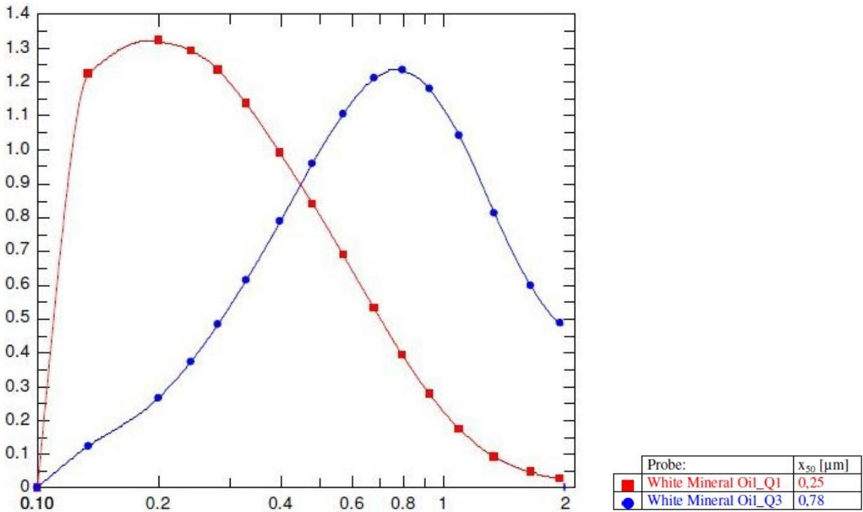
**Figure 4: PDF of particle sizes of white mineral oil atomized at 0.7 bar overpressure**
