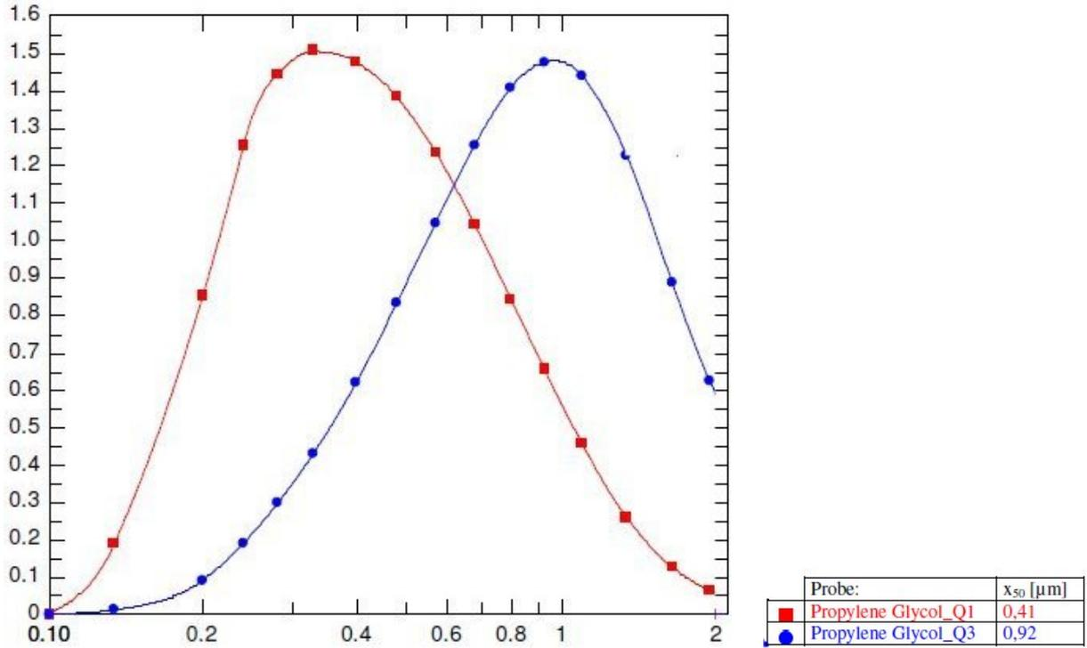
**Figure 5: PDF of particle sizes of propylene glycol atomized at 0.7 bar overpressure**
