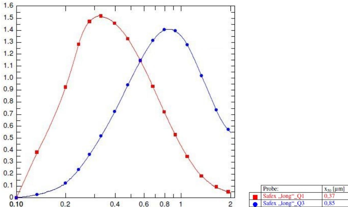
**Figure 6: PDF of particle sizes of Safex “long” fog fluid atomized at 0.7 bar overpressure**
