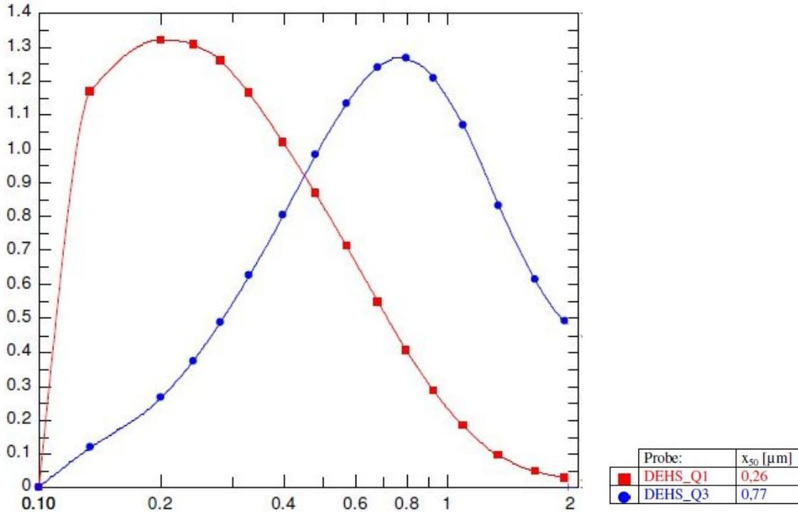
**Figure 3: PDF of particle sizes of DEHS atomized at 0.7 bar overpressure**
