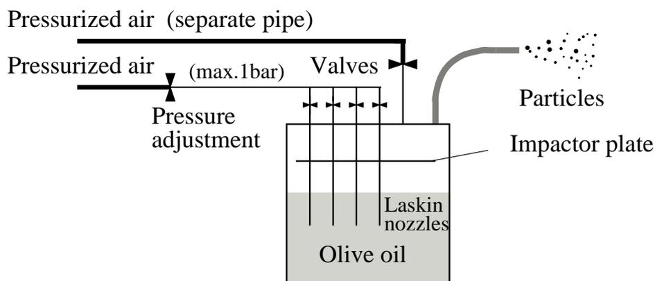
*Figure 1: Principle of the PivPart05 particle generator*
